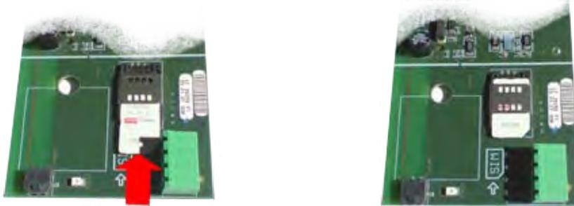
Thereafter, the battery cable (with black connector) is plugged into the matching (black) jack. Thus the device is first started and sends an SMS to the programmed number. This is a first test of the configuration.
